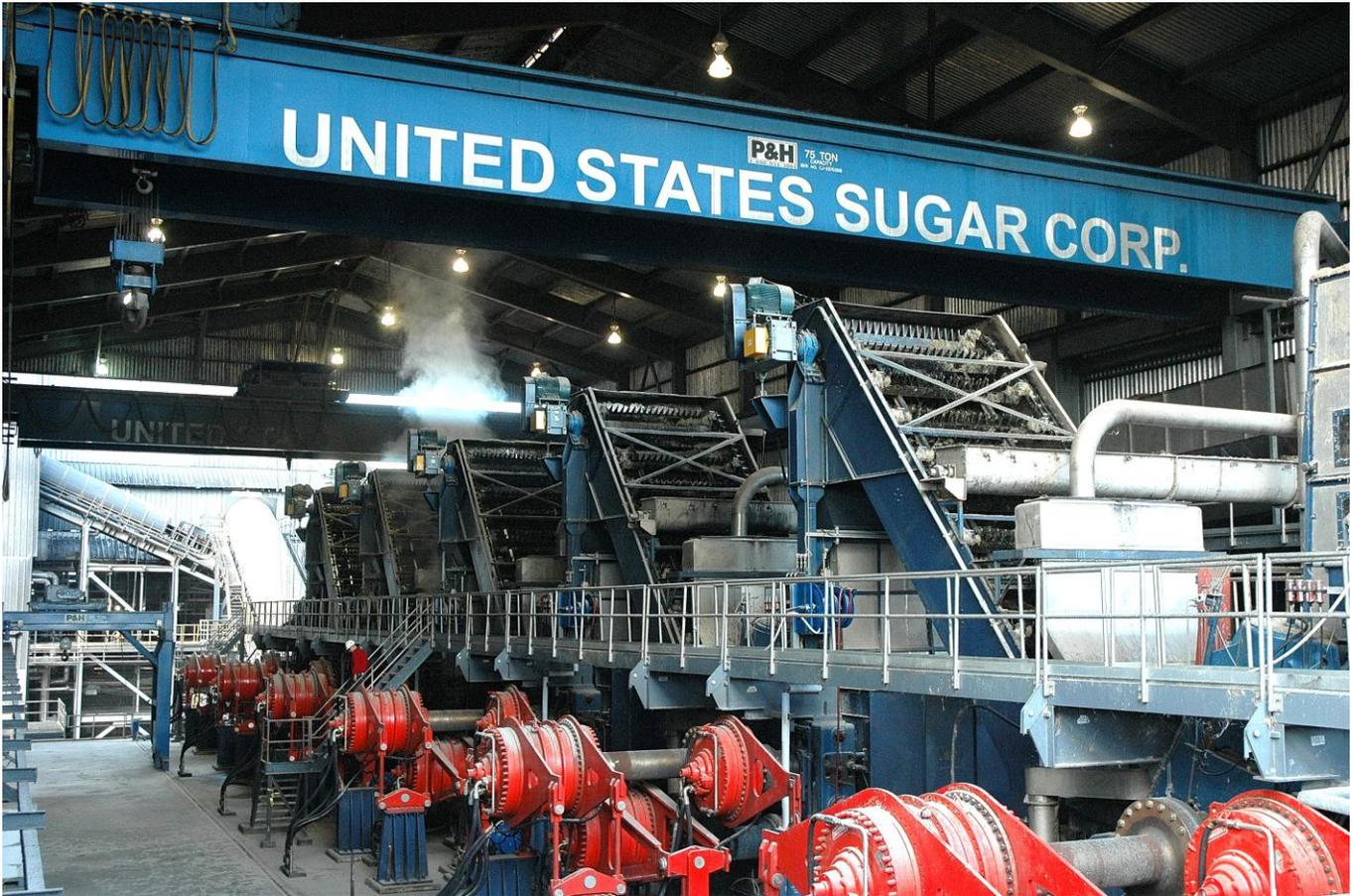
U.S. Sugar's "C-Tandem" can grind 1,575 tons of sugarcane per hour and milled a world-record 4.1 million tons of sugarcane during the 2011-2012 season
