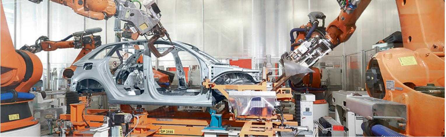
AUDI: High level of automation for assembling the body of the A3
