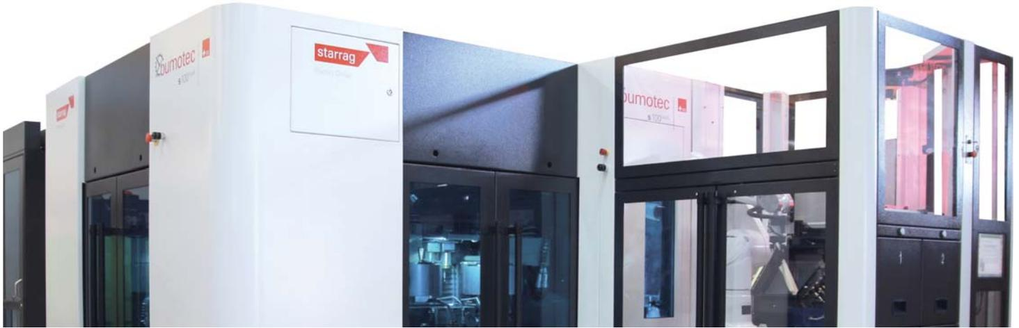
With IndraMotion MTX and IndraDrive, Bumotec realizes high-precision, flexible NC milling center for watch parts
