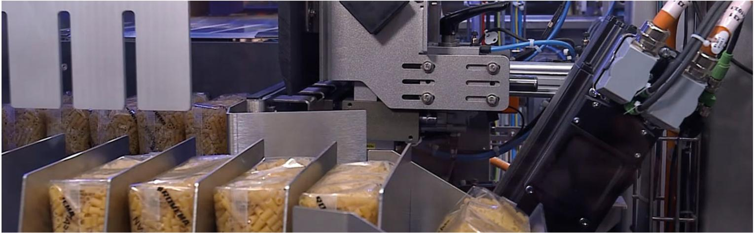
Rovema: Slim machine design based on cabinet-free Rexroth servo technology
