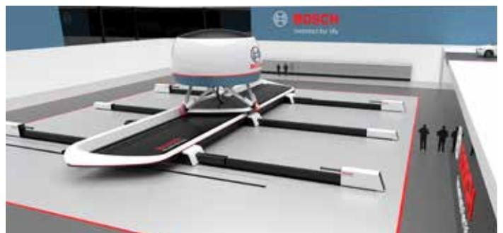
2018 – 6000 kg payload for EX, Korea. First of three similar machines offering higher payloads and large X and Y excursions for complete vehicle testing. Rack and pinion has given way to linear motor technology to deliver the increased accelerations and velocities. The EX system attains 5 m/s velocity, with 0,7G acceleration, while the next system, planned for installation at Renault in 2019, is set to provide 9 m/s velocity with 1G acceleration.
