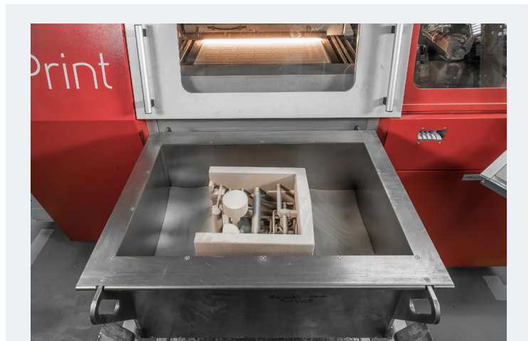
Build envelope with 3D-printed sand core and surplus sand
