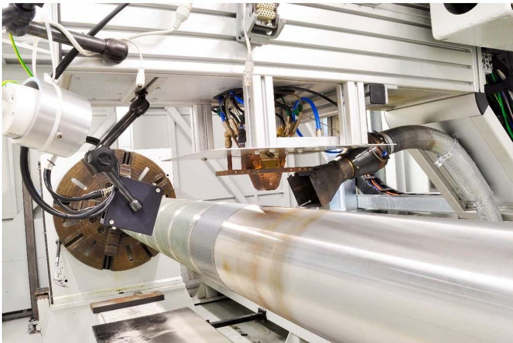
Photo: Laser cladding machine Bosch Rexroth in Boxtel
