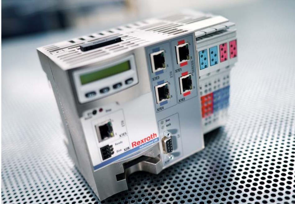
IndraMotion MLC motion logic control for hydraulic drives
