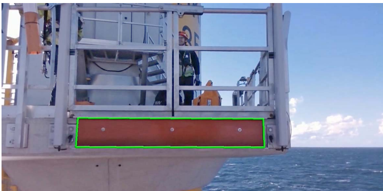
The detection of the docking area is carried video based. (Copyright: Bosch Rexroth AG)
