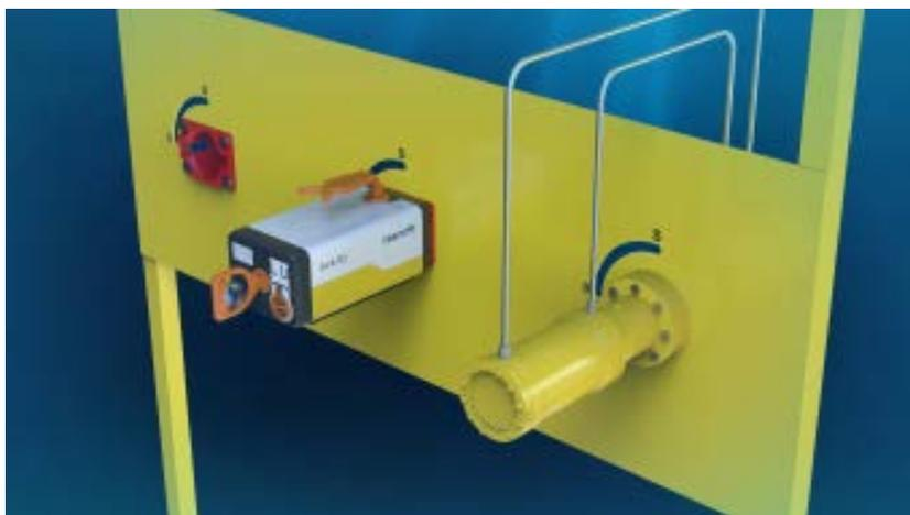
Image 3: The electric Subsea Valve Actuator SVA R2 replaces previously used hydraulic cylinders 1:1 and requires only one cable for power supply and communication. Hydraulic lines several kilometers in length along with the power units and controls are no longer required. (Image source: Bosch Rexroth AG)
